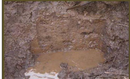
Drainfield Surface Layer Saturation
